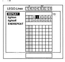
A washing machine manufacturer requires a control program which will rotate the drum one way for 10 seconds and then rotate it the opposite way for 10 seconds. This sequence needs to be repeated 4 times.
