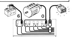
In a drinks dispensing system, a drink is to be pumped out only when a coin has been inserted. Design a program to solve this problem using the LEGO motor as the pump motor and the light brick and opto-sensor as a coin detector.
